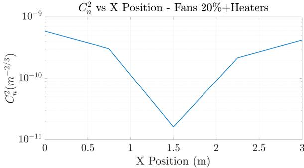
Fig. 5.  $C_n^2$  at different positions in the flow.
