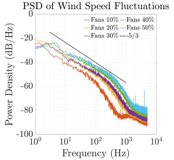
Fig. 3. PSD of WS fluctuations.
