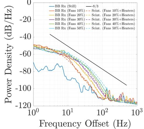
Fig. 7. Measured phase noise versus theoretical scintillation using scaled  $\varepsilon$ .
