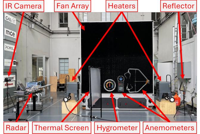
Fig. 2. CAST experimental setup.
