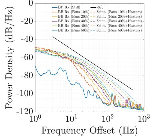
Fig. 6. Measured phase noise vs theoretical scintillation using measured  $\varepsilon$ .
