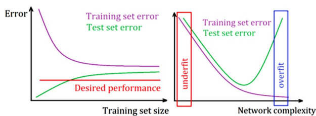
Fig. 8 Left: Example error diagnosis of training a NN model with respect to TS size (Ng 2018). An increase in the size of the TS will not necessarily provide the desired performance. Right: Error diagnosis example of bias vs variance in training a NN model. The underfitting or overfitting (bias vs variance) of a model can be modified based on the network complexity
