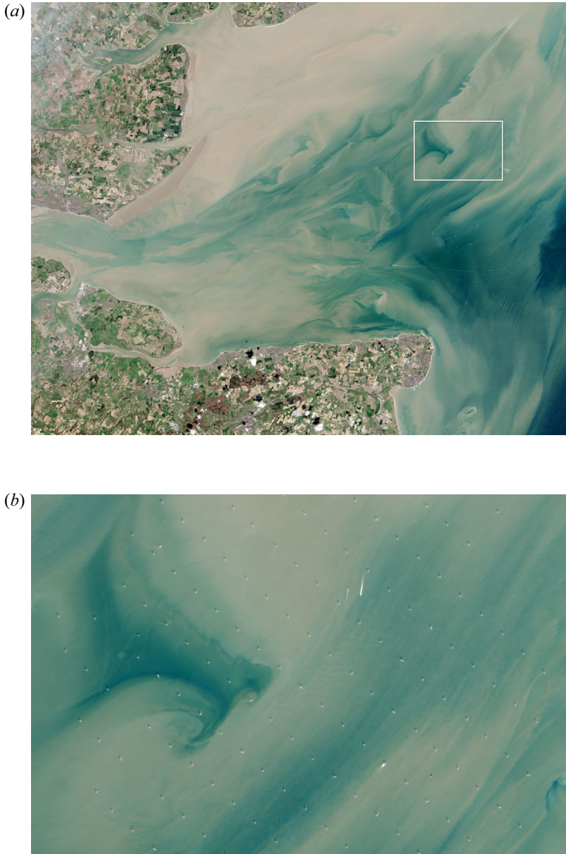
Figure 2. NASA Earth Observatory image by Jesse Allen and Robert Simmon, using Landsat data from the US Geological Survey, showing the offshore wind farm called London Array. (a) The offshore wind farm located in the Thames estuary (the stem array is in the rectangular zone). (b) Enlargement of the stem array of the wind farm.
