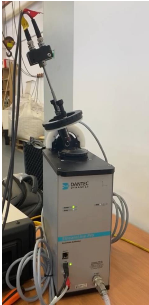
Figure 4.12 Dantec Dynamics calibrator with the two x-probe holder.
