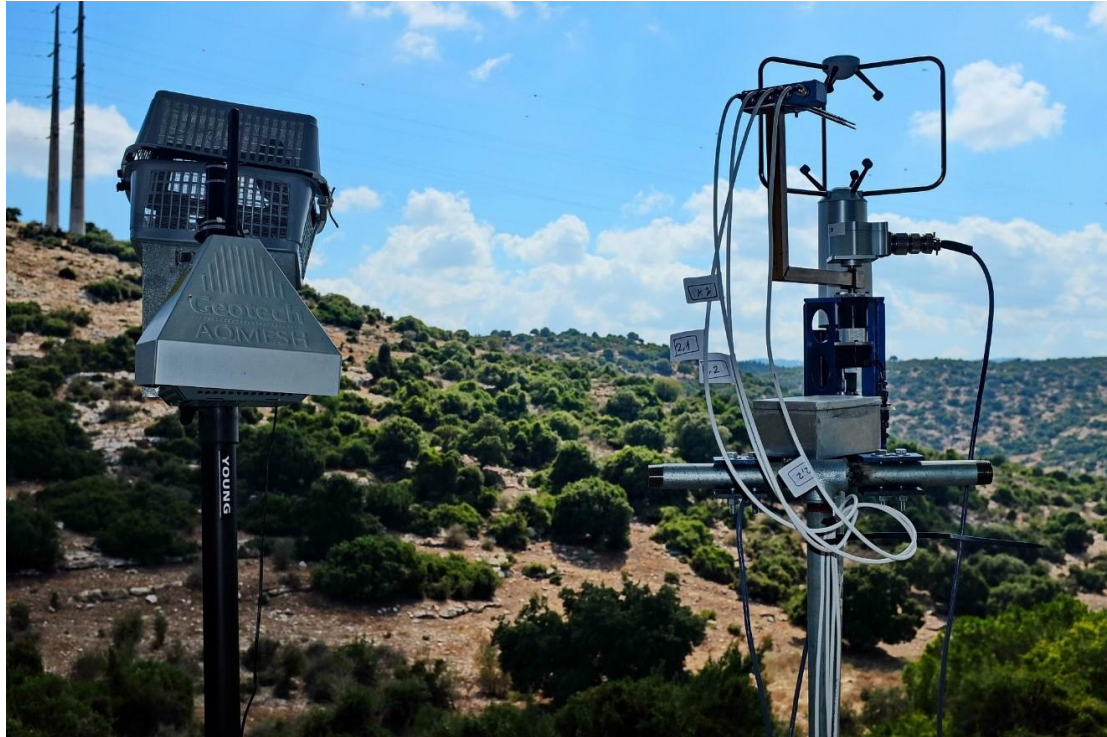
Figure 2.3 Two measuring instruments on the left side of the image are the AQMesh (pyramid shaped device) and inside the plastic cage is the laser particle counter; on the right side of image is the Combo including: Ultrasonic Anemometer and two X-shaped hot film probes.
